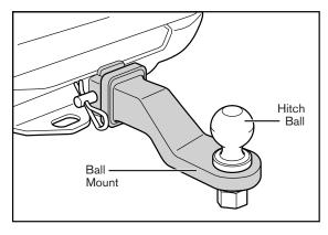
To keep the hitch ball in top condition, a simple maintenance routine is recommended. Coating it with light grease will minimize wear of both the coupler and hitch ball. In addition, removing the hitch ball when not towing, or protecting it with a special cover will help prevent rust from forming on it.
