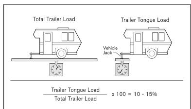
jack is placed directly under the trailer tongue coupler, and the tongue is set at the height/level of the tow vehicle hitch.
