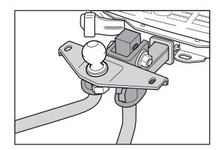
weight-distributing hitch ball mount (Class IV) is recommended if you plan to tow trailers with a maximum weight over 5,000 lbs. This ball mount includes a 2-5/16" hitch ball and is available through your NISSAN dealer.
