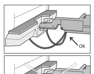
A WARNING- DO NOT use S-hooks for attaching the safety chains as they may become un-hooked while towing. If the S-hook unhooks, the emergency chains/cables will become detached, so if the tow hitch breaks or becomes disengaged, it will allow the trailer to completely break away causing property damage and possibly personal injury or death. The use of S-hooks is illegal in many states.
