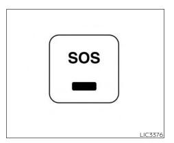
The Emergency call (SOS) system button used in combination with a NissanConnect® Services subscription to call for assistance in case of an emergency.
