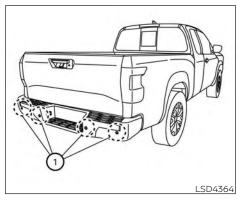
The RAB system detects obstacles behind the vehicle using the parking sensors ① located on the rear bumper.
