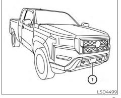
The I-FCW system uses a radar sensor ① located on the front of the vehicle to measure the distance to the vehicle ahead in the same lane.
