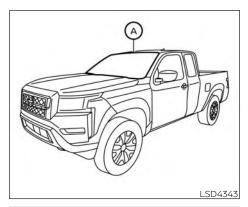
The LDW system will operate when the vehicle is driven at speeds of approximately 37 mph (60 km/h) and above, and only when the lane markings are clearly visible on the road.
