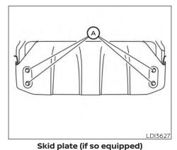
Removal of under-engine protectors
