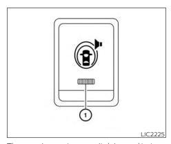
The warning systems switch is used to turn on and off the following systems that are activated using the Settings menu in the vehicle information display:
