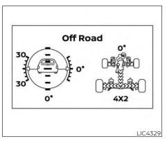
The Tire Angle & 4WD Gauge (right) indicates the angle of the tires based on turning of the steering wheel and 4WD status. The graphic image will show the actual vehicle tire position while the angle is to be displayed above as reference. The 4WD status is displayed below.
