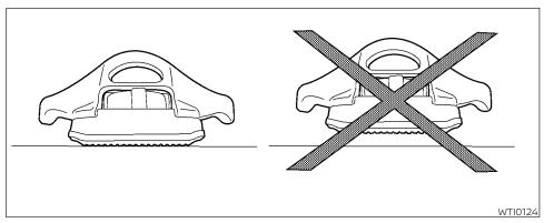
5. There should be no gap between the bottom of the cleat and the top of the channel. Tighten the center bolt hand tight 20-40 in-lbs. (2.27 - 4.6 N·m).
