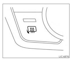
To defrost the outside mirrors, start the engine and push the outside mirror defroster switch on. The indicator light on the switch will illuminate. Push the switch again to turn the defroster off.
