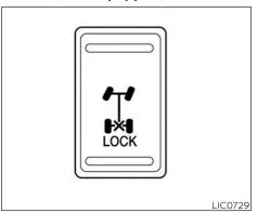
The E-Lock system can help provide added traction if the vehicle is stuck or becoming stuck
