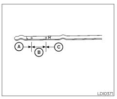
5. Remove the dipstick again and check the oil level. It should be between the H (High) and L (Low) marks (a). This is the normal operating oil level range. If the oil level is below the L (Low) mark (a), remove the oil filler cap and pour recommended oil through the opening. **Do not overfill** (a).
