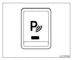
The Parking Aids system switch on the instrument panel allows the driver to turn the following systems (if so equipped) on and off. To turn the systems on and off, the ignition switch must be in the ON position.
