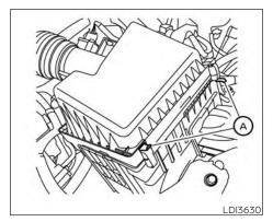
The dry paper type filter element may be cleaned and reused. Replace it according to the maintenance log shown in the "Maintenance and schedules" section of this manual.
