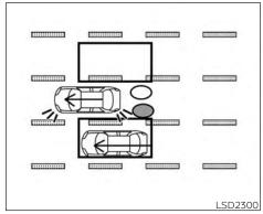
Illustration 2 - Approaching from behind Illustration 2: If the driver activates the turn signal when another vehicle is in the detection zone, then the system chimes (twice) and the side BSW/RCTA indicator light flashes.
