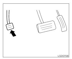
To engage: Firmly depress the parking brake.
