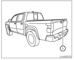
To display the rear view, the Rear View Monitor system uses a camera located just above the vehicle's license plate ① on the tailgate.
