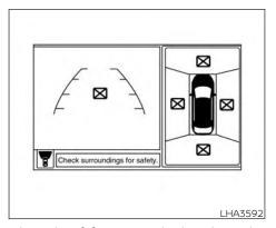
When the "[X]" icon is displayed on the screen, the camera image may be receiving temporary electronic disturbances from surrounding devices. This will not hinder normal driving operation but it is recommended that the system be inspected if it occurs frequently. It is recommended that you visit a NISSAN dealer for this service
