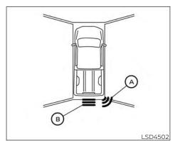
When the corner of the vehicle moves closer to an object, the corner sonar indicator (A) appears. When the center of the vehicle moves close to an object, the center sonar indicator (B) appears.
