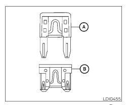
Two types of fuses are used. Type (A) is used in the fuse boxes in the engine compartment. Type (B) is used in the passenger compartment and engine compartment fuse boxes. Type (A) fuses are provided as spare fuses. There are no spare fuses in the engine compartment.
