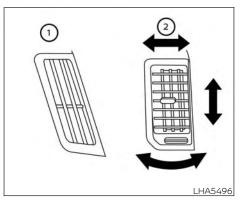
Adjust air flow direction for the driver and passenger's side vents or center vents ② by moving the vent slide and/or vent assemblies. Open or close the driver, passenger and center vents by using the dial. The defrost vents ① located above the driver and passenger side vents cannot be adjusted or closed.
