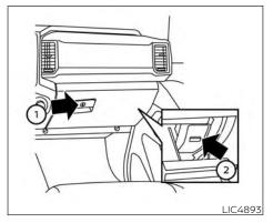
The extended storage switch is used when shipping the vehicle. It is located in the fuse panel inside the glove box. To reach it, open the glove box 1 on the instrument panel, then open the fuse panel cover ②.
