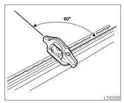
3. Insert the cleat into the channel perpendicular to the channel as shown. Then rotate the cleat clockwise 90° and slide it to the desired location.
