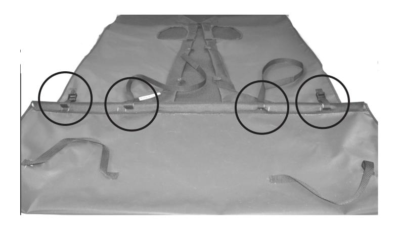
Once the bar is in place you can put the liner in place with the back seats down. (Once this installation is done we will show you how install it with the back seats up.) There are two straps sewn to the back side of the cargo liner. These two straps loop around the rear seat head rest as shown. The two straps around the top go around the front seat head rest and connect to the cam lock.
