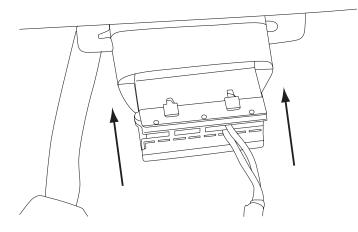
4 Mount the microphone as illustrated and run the cable to the radio cavity. You will need to use a T20 Torx to remove the visor. For optimal performance it should be mounted by the rear-view mirror as illustrated.
