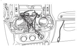
2 Plug the OBDII connector on to the OBDII port below the driver side dash and run the extension to the radio cavity.
