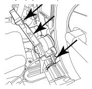
5 Extract (4) 7 mm screws and remove the factory radio.
