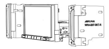
For 2011-2017 vehicles: For vehicles with uConnect refer to page 11. For vehicles without uConnect run the USB extension cable to the glove box, connect the main harness, antenna, and other adapters to the factory harnesses and secure them. Route all cables through the lower opening of the rear support bracket as shown below.
