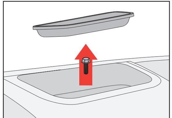
3. Install Accessory Mount Base. Hooks on arms of Accessory Mount Base will snap into upper dashboard vents closest to windshield.
