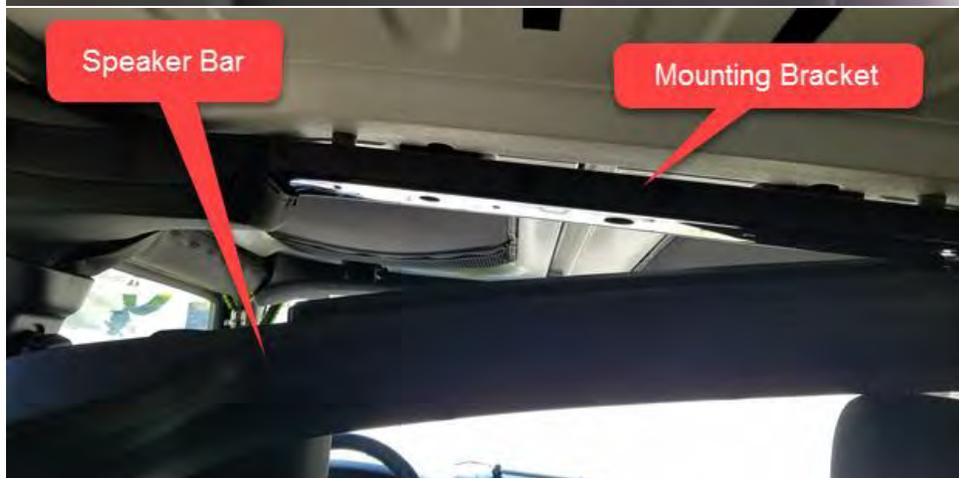
7. Lastly make sure that each piece has been firmly pushed in place so that they don't fall while operating the vehicle.
